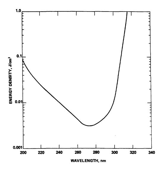
Figure I-1. Recommended Ultraviolet Radiation Exposure Standard This figure was adapted from a figure developed and published by the American Conference of Governmental Industrial Hygienists in "Threshold Limit Values for Chemical Substances and Physical Agents in the Workroom Environment with Intended Changes for 1972".
